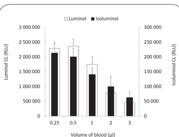
**Figure 1.** Effect of blood volume on luminol- and isoluminol-enhanced chemiluminescence (CL) of human whole blood. Samples (250  $\mu$ l) contained from 0.25 to 3  $\mu$ l of blood, HRP (8 U/ml), luminol or isoluminol (100  $\mu$ mol/l). Chemiluminescence was recorded continuously for 60 min at 37°C. Columns represent mean integral values of chemiluminescence (area under chemiluminescence curve). Mean  $\pm$  SEM, n=4–8, RLU – relative light units.
