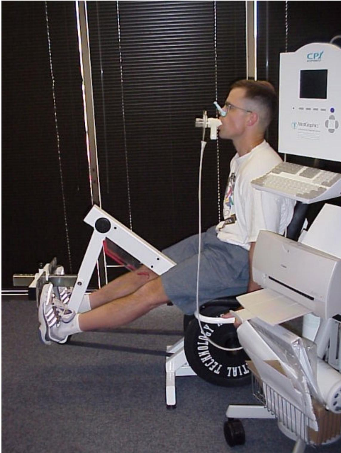
**Figure 2.** Configuration of the prototype flywheel ergometer and metabolic cart as current study seated calf press repetitions were performed.
