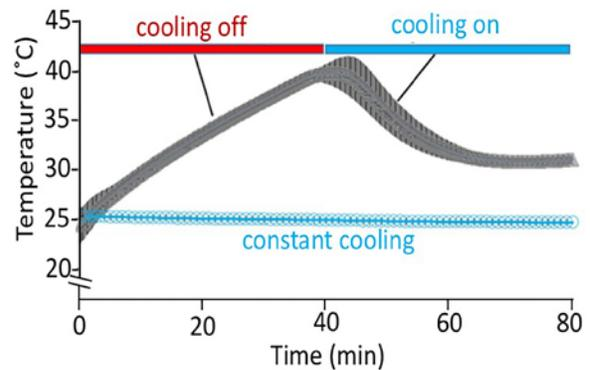
**Figure 4.** Temperature profiles recorded below the far-red light treatment device. Data represent mean  $\pm$  SEM,  $n=3$ . Upper trace, stress test for local heat buildup, with the liquid cooling system being activated at 40 min. Lower trace, temperature below the light rail with the liquid cooling system running continuously.
