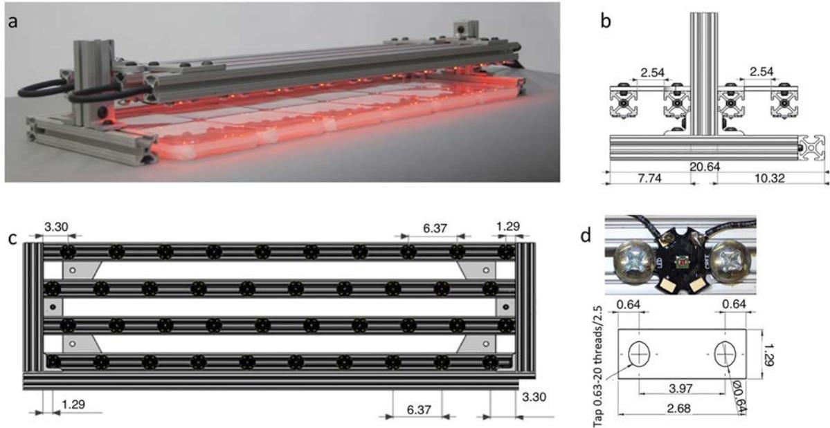
**Figure 3.** Far-red illumination system (a), side view (b), bottom view showing the alternating alignment of the LEDs (c), and mounted LED viewed from under side and custom steel nut (d). CAD drawings for the extruded aluminum and connectors are from the manufacturer. Dimensions in cm unless noted otherwise.
