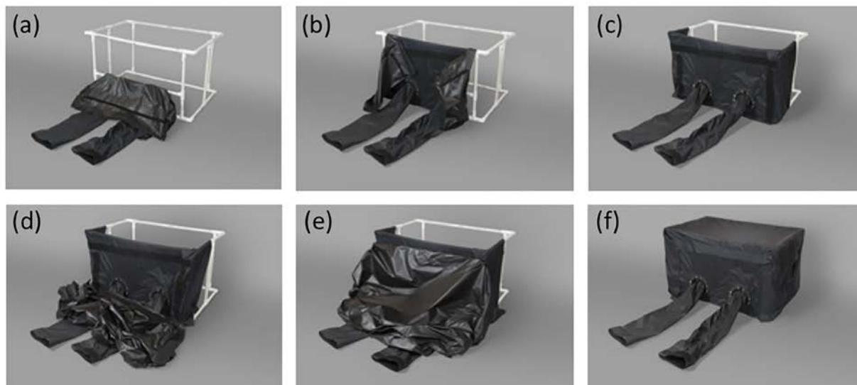
**Figure 2.** (a-f) Assembly of the portable benchtop darkroom. The tent covers the PVC frame with integral sleeves to allow access to the Petri dishes to be irradiated inside without interference from ambient room lights. Dimensions are 93 cm×62 cm×62 cm.
