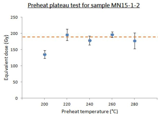
**Fig. 5.** Preheat plateau test for sample MN15-1-2, with a  $D_e$  plateau obtained for preheat temperatures from 220°C to 280°C.
