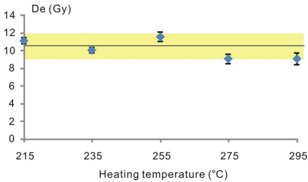
Fig. 4. The SAR-ITL protocol dose recovery test results.
