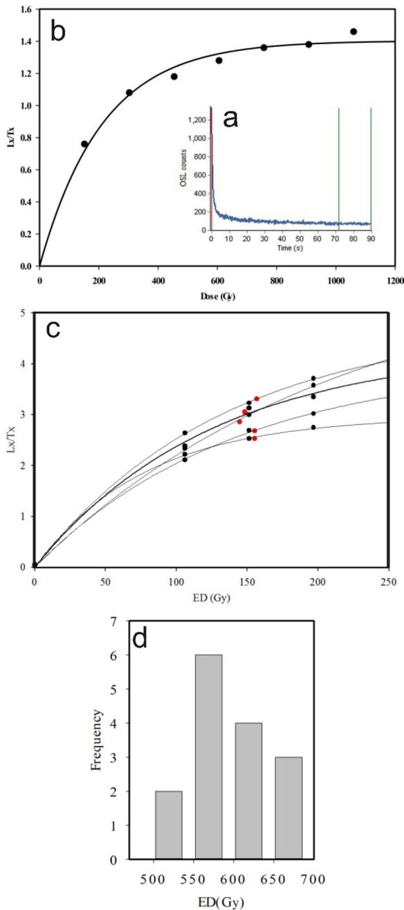
**Fig. 4.** (a) The BSL shine down curve for the quartz from the JRM-1 sample. (b) The laboratory generated dose growth for the sample JRM-1. (c) The dose recovery test was performed on the S-5, laboratory dose of 151.4 Gy was administered and it was recovered, the red dots represent the recovered doses. It was found that all the five aliquots showed very good recovery with less than 10% of deviation from the given lab dose. (d) Histogram showing the dose distribution for the sample JRM-1.
