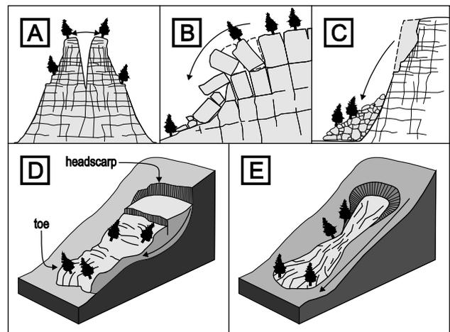
Fig. 1. Types of mass-movements with the location of trees affected (possibly recording the geomorphic impact): A – lateral spreading, B – toppling, C – rock fall, D – landslide, E – debris flow.
