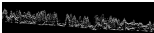
Fig. 1. A typical profile of Smolnícka Osada model forest derived from airborne laser scanning data.
