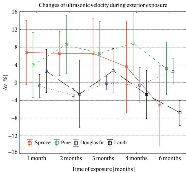
Fig. 2. Two sides confidence intervals of Δv in softwood species during exterior exposure.
