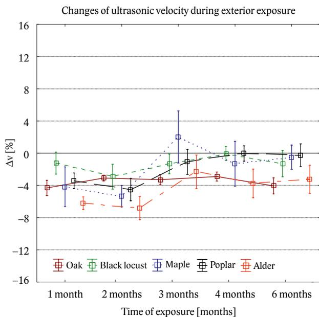
Fig. 3. Two sides confidence intervals of Δv in hardwood species during exterior exposure.
