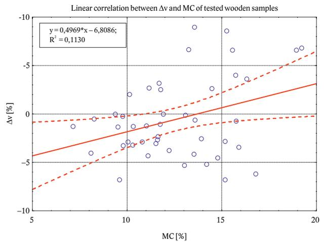
Fig. 5. Correlation between Δv and MC for all tested wood.
