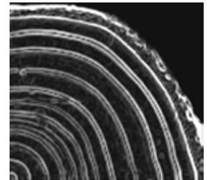
**Fig. 3.** Magnification of detail: A spruce disc after application of the standard Sobel operator illustrates double edges which can occur with wide late wood parts.
