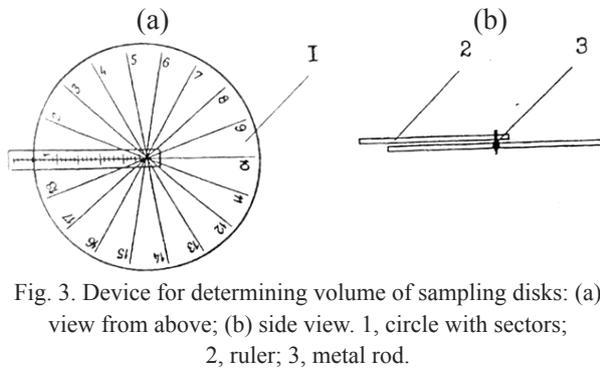
Fig. 3. Device for determining volume of sampling disks: (a) view from above; (b) side view. 1, circle with sectors; 2, ruler; 3, metal rod.
