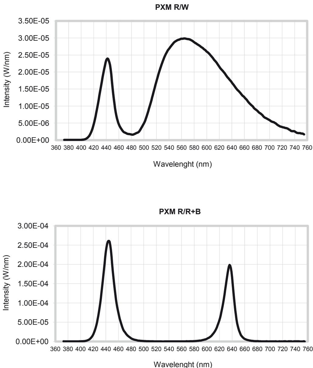
**Figure 1.** Spectral distribution of the LED lamps used in this study: R/W emitted white light and R/R+B emitted red and blue light. This characteristic was measured at a distance of 40 cm under the lamp (on the plant level when photosynthesis parameters were measured)
