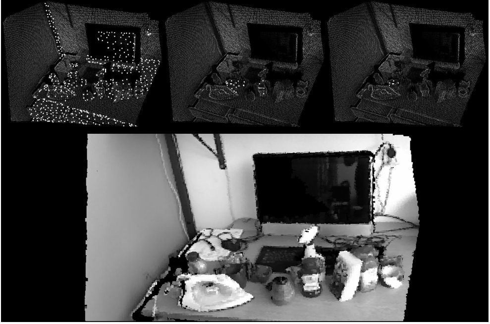
Figure 3. Example test scene from our Kinect Fusion dataset processed in the proposed hierarchical manner. The white dots represent the anchoring points for (from left to right) non-flat filtering, ICAHSD and Combined descriptor classification for the task of cup detection. An additional view of RGB colors converted to grayscale is provided.
