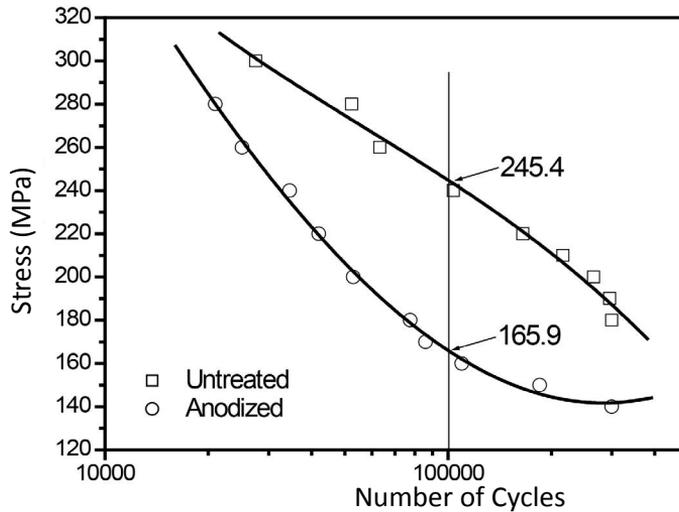
Fig. 3. S-N curves for 2024-T-351-aluminum alloy: (i) without anodizing, and (ii) anodized (batch 4)
