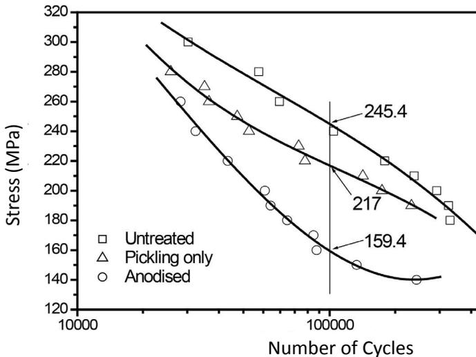
**Fig. 2. S-N curves for 2024-T-351-aluminum alloy: (i) without anodizing, (ii) pickling treatment and (iii) anodized (batch 3)**
