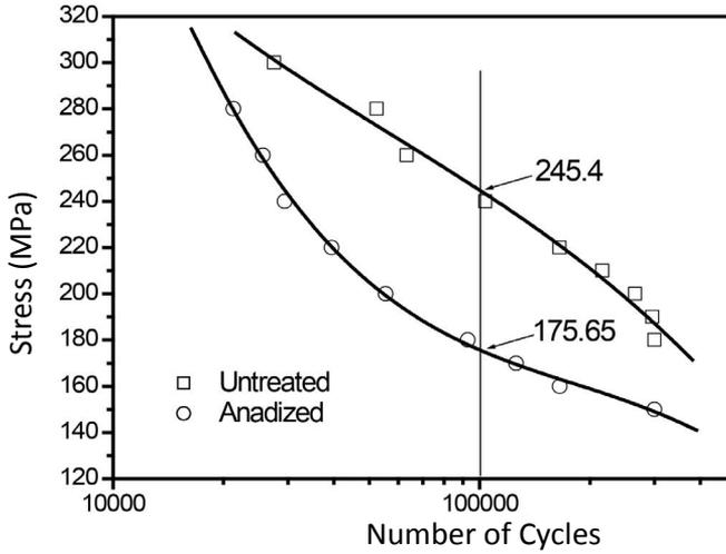
**Fig. 4. S-N curves for 2024-T-351-aluminum alloy: (i) without anodizing, and (ii) anodized (batch 6)**
