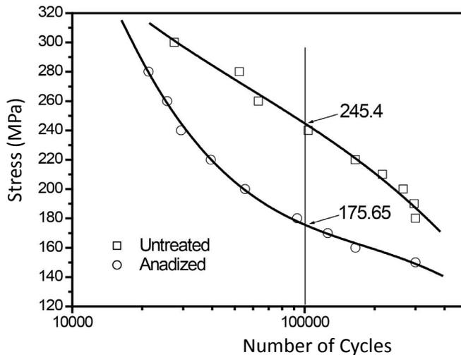
Fig. 4. S-N curves for 2024-T-351-aluminum alloy: (i) without anodizing, and (ii) anodized (batch 5)
