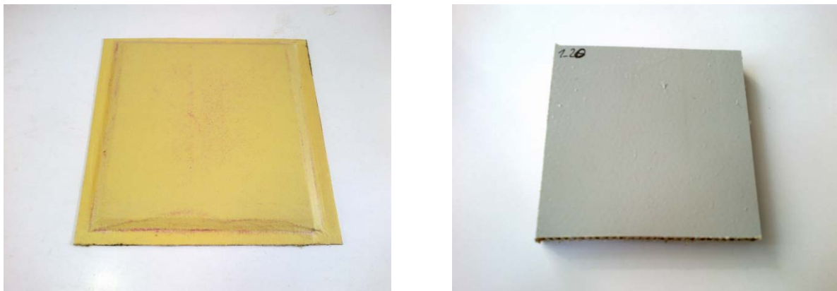
Figure 2. Honeycomb panel after curing (left), one of the specimens (right)
