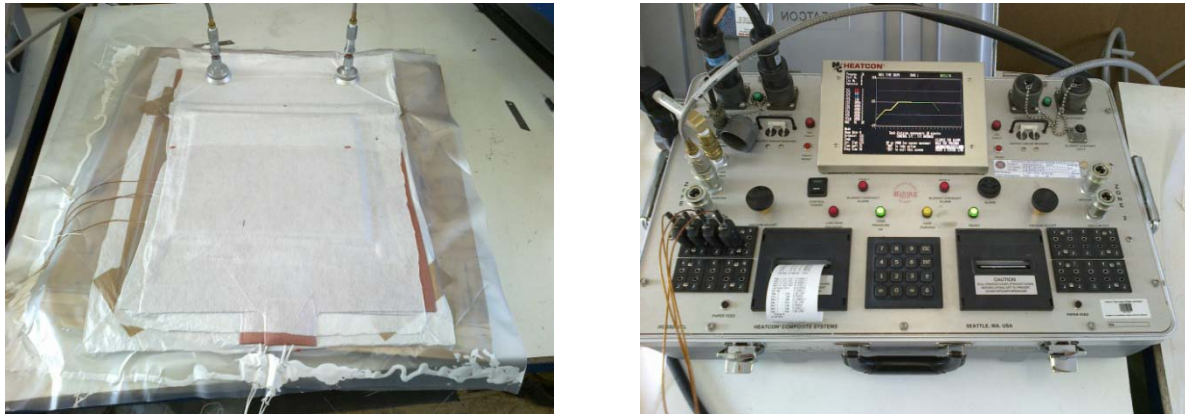
Figure 1. Honeycomb panel during curing cycle
