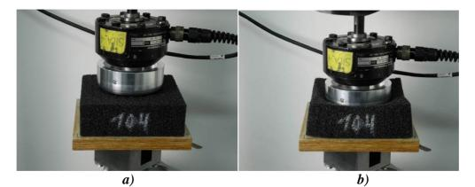
Fig. 2. Indenter and S28280 auxetic foam sample: a) before the test, b) during 40,000 cycle [6]
