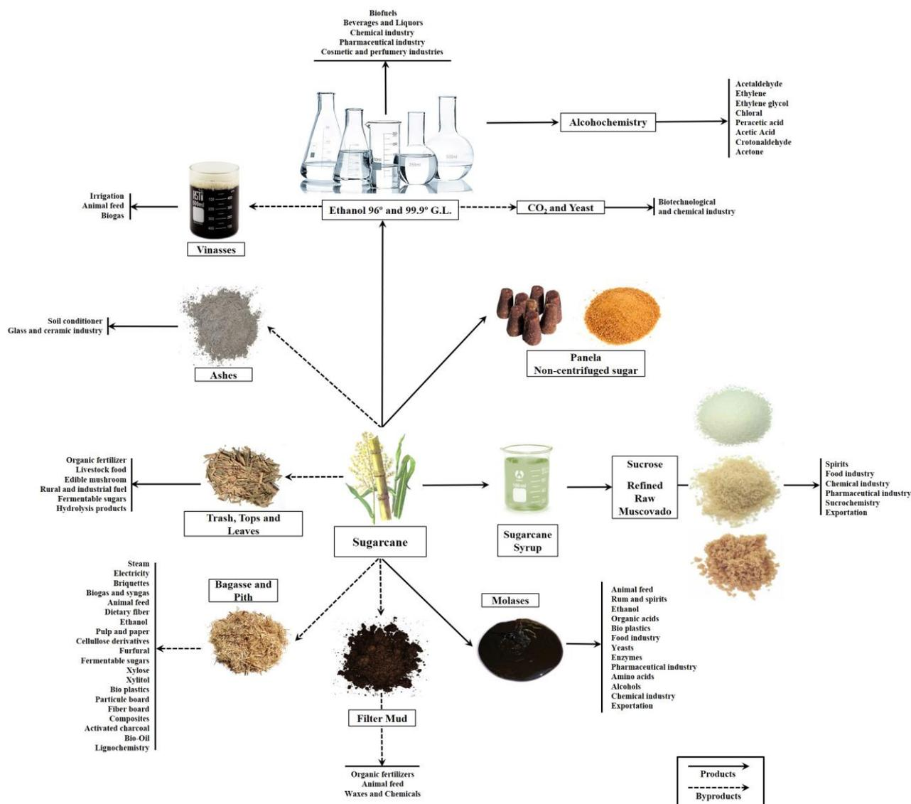
Fig. 1. Sugarcane biorefinery based on cane, products and byproducts
