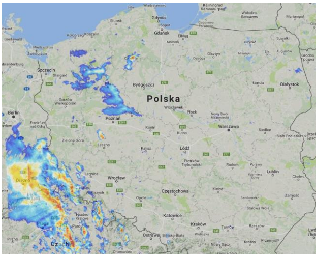
A) CAPPI (1 km) showing reflectivity at the height of 1 km at 14:00 UTC. Convective system is located in the Czech Republic and the new storm cells are developing over the Sudety Mts.
