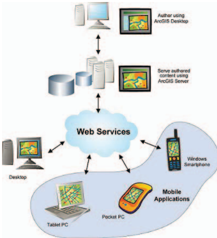
Fig. 7. Client/server architecture of a web-based geodata management and monitoring system ( www.mapping.com/mobileanwendungen ).
