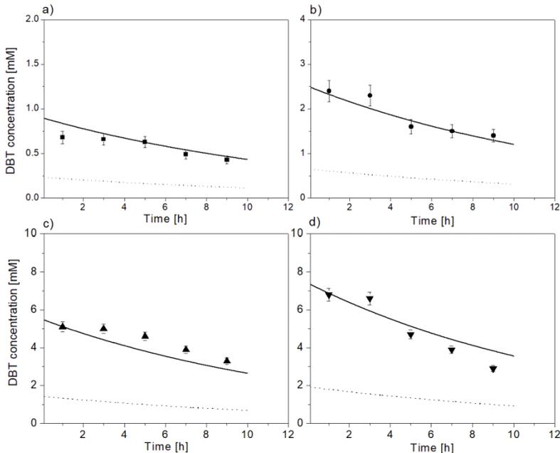
Fig. 3. Comparison of variation in DBT concentration with reaction time for BDS reaction experiments, in adsorbed bacterial cells system with different initial DBT concentrations in bulk liquid ( $DBT_o$ ) (1 mM (■), 3 mM (●), 5 mM (▲) and 7 mM (★) and modelling predictions (—). The dashed lines (---) correspond to  $DBT_s$  concentration in the film surrounding the particle surface ( $DBT_s$ ). Data are mean values of three independent assays. Error bars show the standard deviation
