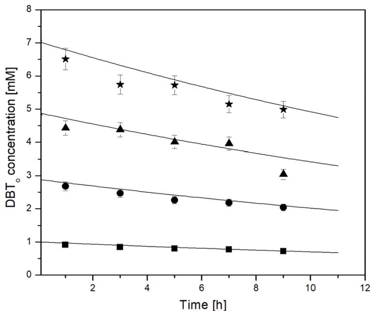
Fig. 2. Comparison of variation in DBT concentration with reaction time for BDS reaction experiments, in suspended bacterial cells system with different initial DBT concentrations in bulk liquid (DBT<sub>o</sub>) measured (A = 1 mM (■), B = 3 mM (●), C = 5 mM (▲) and D = 7 mM (★)) and the results of first order modeling (—). Data are mean values of three independent assays. Error bars show the standard deviation
