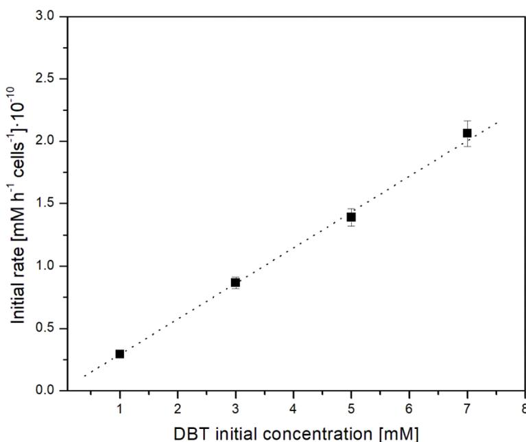
Fig. 1. Initial rate versus initial DBT concentration in suspended bacterial cells system. Data are mean values of three independent assays. Error bars show the standard deviation
