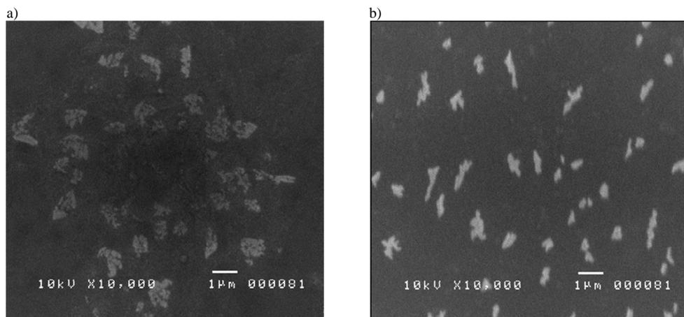
Fig. 7. SEM micrographs of the synthesized silver nanoparticles by Isolate nos. 9 (a) and 14 (b)
