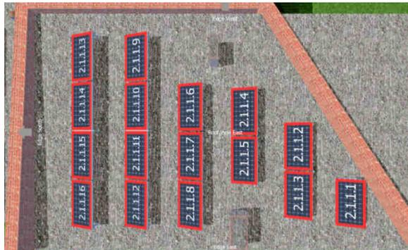
Fig. 5. Deployment of photovoltaic panels, Section 3 (red) 16 modules on the upper part of the roof [14]
