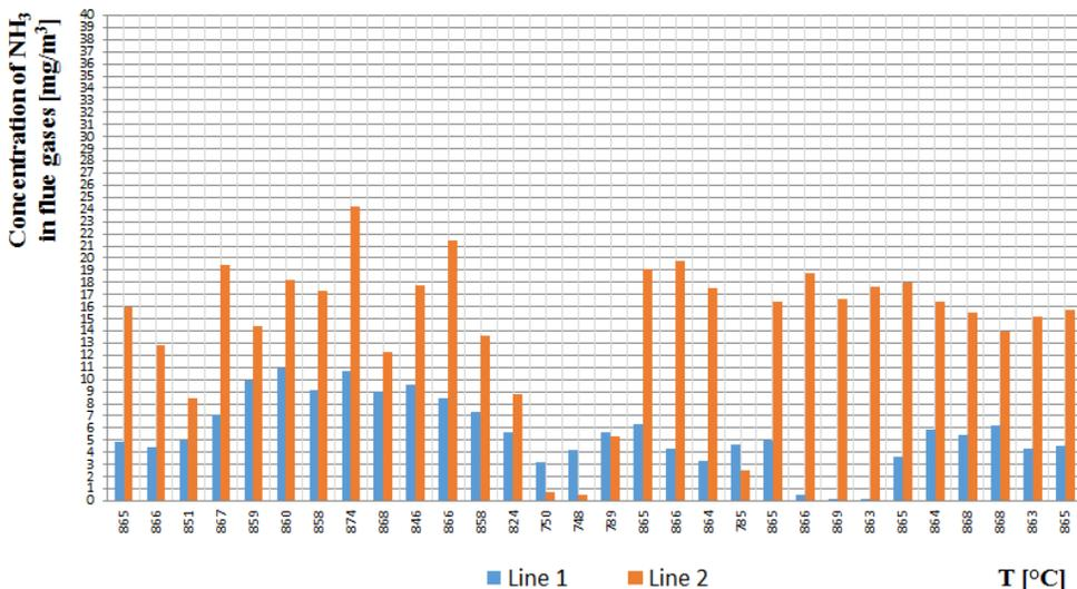
Fig. 4. Ammonia emission from a sewage sludge incineration plant - concentrations of  $\text{NH}_3$  in flue gases in function of temperature measured in April 2014
