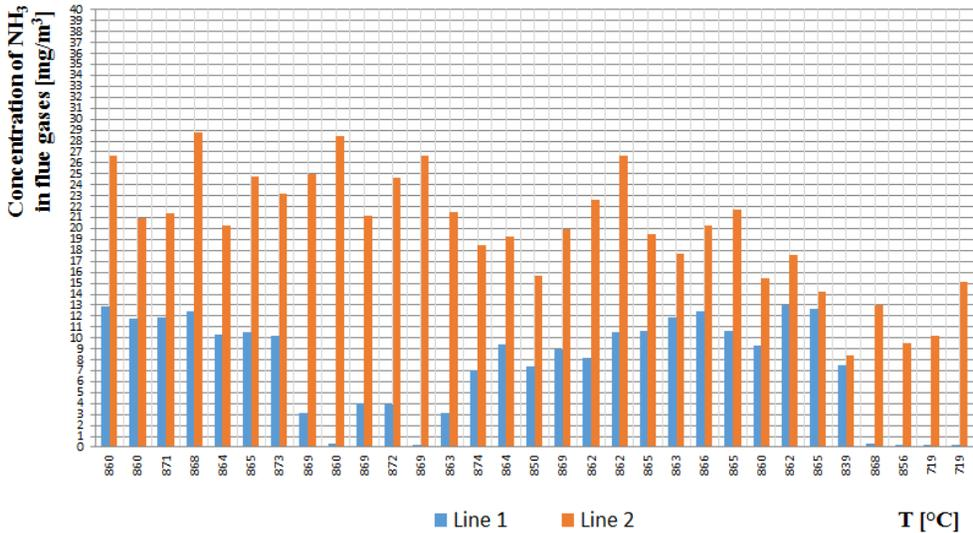
Fig. 5. Ammonia emission from a sewage sludge incineration plant - concentrations of  $\text{NH}_3$  in flue gases in function of temperature measured in October 2014
