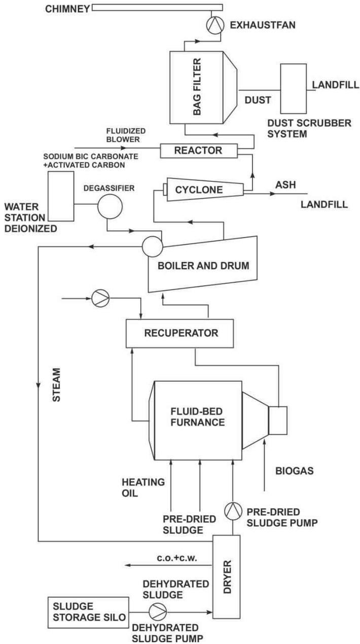
Fig. 3. Schematic diagram of Sewage Sludge Incineration System in GOS Lodz Ltd.
