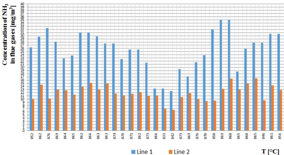
Fig. 6. Ammonia emission from a sewage sludge incineration plant - concentrations of  $\text{NH}_3$  in flue gases in function of temperature measured in December 2014
