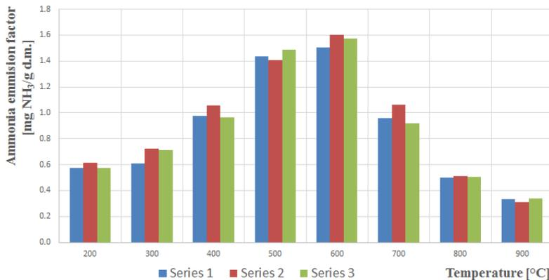
Fig. 8. Ammonia emission factor (per combusted sludge mass) as a function of combustion temperature
