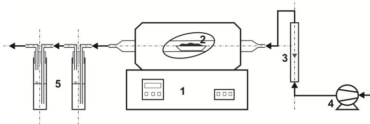
Fig. 7. Schematic diagram of the experimental set-up: 1 - electrical furnace with quartz tube, 2 - examined sample, 3 - rotameter, 4 - air pump, 5 - glass scrubber
