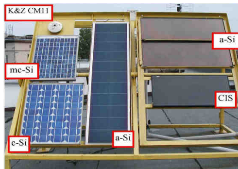
Fig. 1. Research station to test PV modules in the outdoor conditions. View from 2002
