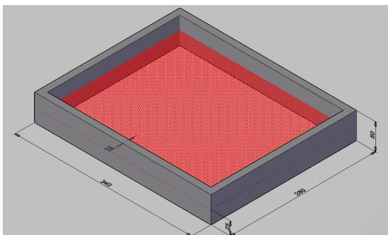
Fig. 2. Image of the wooden frame
