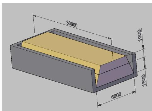
Fig. 3. Schematic representation of the composting clamp
