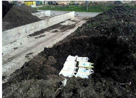
Fig. 4. Placement of samples in the compost pile
