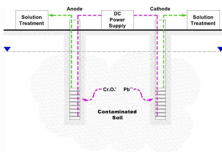
Fig. 4. Electrokinetic technology for heavy metal contamination remediation
