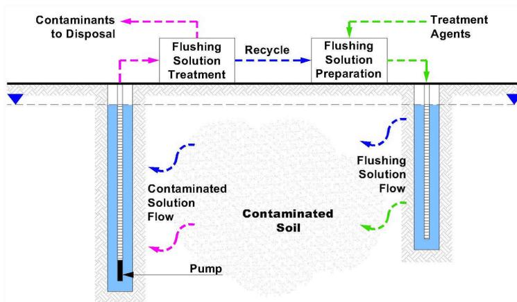
Fig. 3. Soil flushing technology
