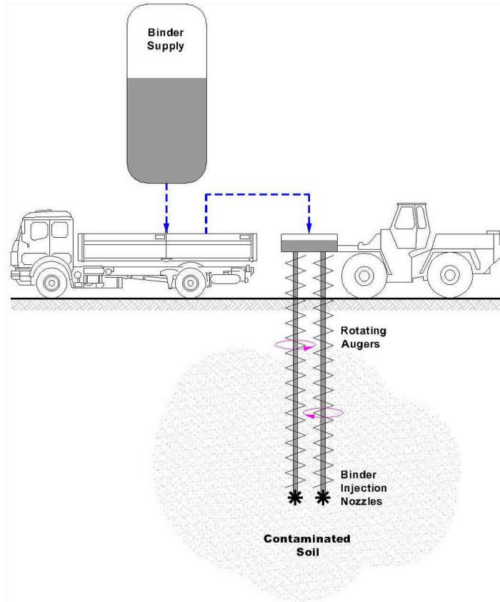
Fig. 2. Stabilization/solidification technology for remediation of various contaminants - heavy metals, oil products, PCB's etc.
