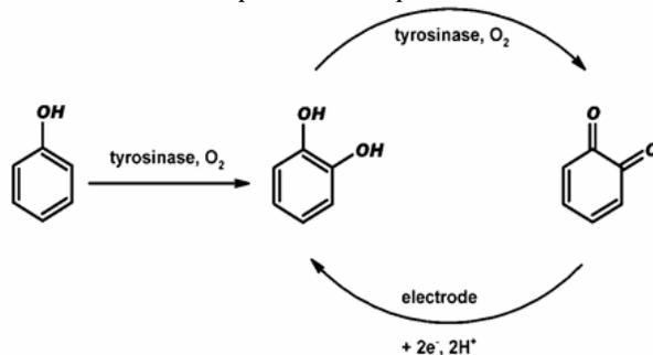
An amperometric biosensor based on tyrosinase immobilized in titania sol-gel has been proposed [22]. The developed biosensor shows high sensitivity towards phenolic compounds (catechol, phenol, *p*-cresol, *p*-chlorophenol and *p*-methylcatechol), low limit of detection ( $0.012 \text{ mg/dm}^3$  for phenol) and satisfying linear range ( $0.04 \div 1.03 \text{ mg/dm}^3$ ).
