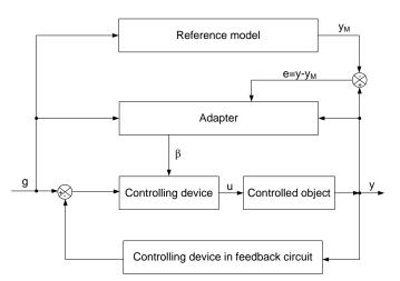
Fig. 5. Structural scheme of adaptive system with reference model.
