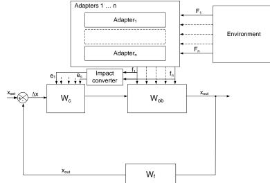
Fig. 6 Structural scheme of adaptronic system.
