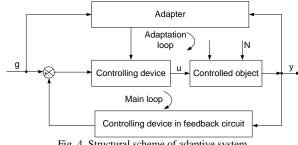
Fig. 4. Structural scheme of adaptive system.
