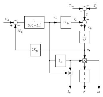
Fig. 5. Modified model of PM BLDC motor, taking into account the impact of inductance.
