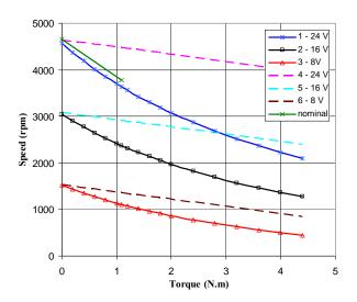
Fig. 9. Torque-speed characteristics of the motor obtained by computer simulations for three supply voltage values (24V, 16V and 8V): 1, 2, 3 - characteristics for modified constant current model, 4, 5, 6 - characteristics for non-modified constant current model, 7 - nominal working point.
