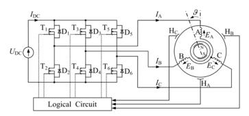
Fig. 1. Electrical connections scheme for 3-phase, 2-pole PM BLDC motor.
