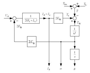
Fig. 4. Constant current model of PM BLDC motor.
