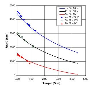
Fig. 10. Torque-speed characteristics of the motor obtained by computer simulations of modified model (1, 2, 3) for three supply voltage values (24V, 16V and 8V), with additional resistance  $R_{ad} = 0.04 \Omega$  and additional inductance  $L_{ad} = 0.01$  mH; measurement results (4, 5, 6) obtained for identical voltages.
