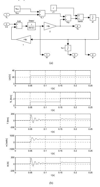
Fig. 6. Constant current computer model of PM BLDC motor: (a) scheme, (b) waveforms of supply voltage  $U_d$ , load torque  $T_{L_3}$  electromagnetic torque T, angular velocity  $\omega$  and motor current  $I_d$ .
