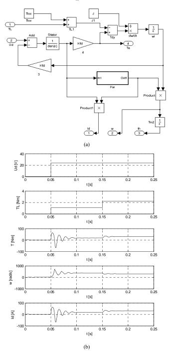
Fig. 7. Modified computer model of PM BLDC motor with inductance impact taken into account (a) scheme, (b) waveforms of supply voltage  $U_d$ , load torque  $T_L$ , electromagnetic torque T, angular velocity  $\omega$  and motor current  $I_d$ .
