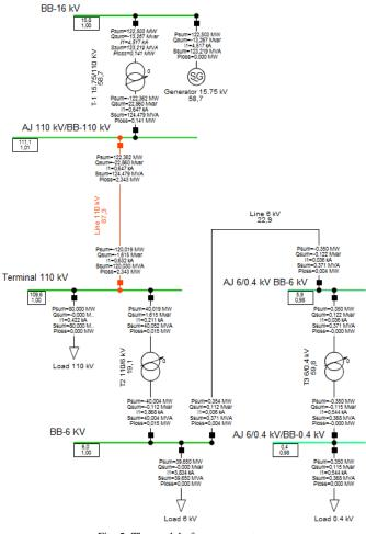
Fig. 5. The model of a power system.
