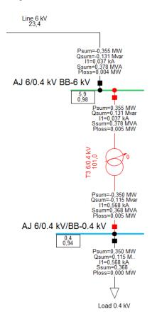
Fig. 4. PFS demonstrating the influence of reactive power on the equipment capacity.
