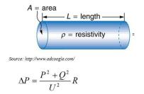
$\Delta P$  – active power losses in conductor, MW
