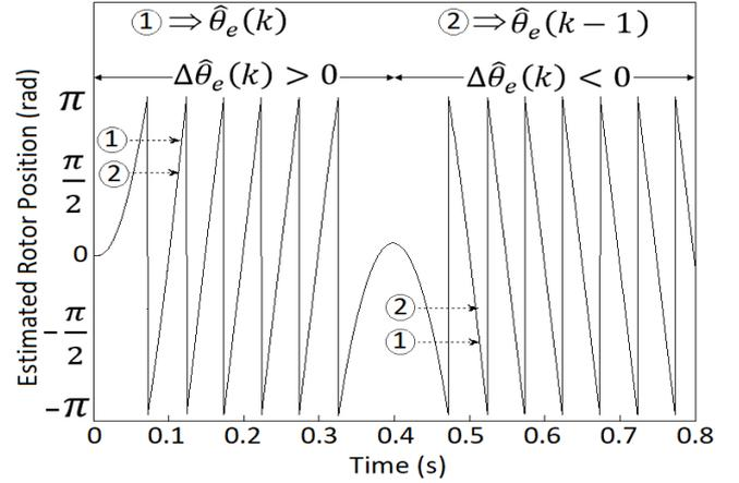
Fig. 2. Estimated rotor position for different step change in reference speed.
