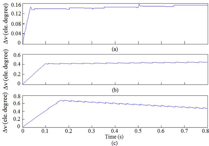
Fig. 13. Estimated rotor position error when step change in load torque from no-load to 10 N m and from 10 N m to  $-10$  N m with reference speed set at (a) 100 rpm (b) 300 rpm and (c) 500 rpm.
