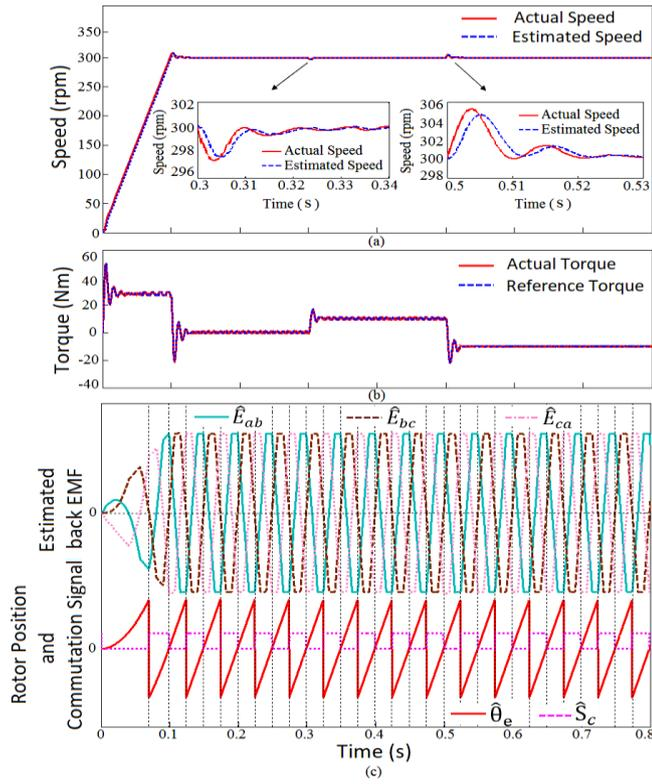
Fig. 9. Dynamic response of (a) speed (b) torque and (c) ZCP of back EMF, rotor position and commutation signal for step change in load torque from no-load to 10 Nm and from 10 Nm to -10 Nm with reference speed set at 300 rpm.
