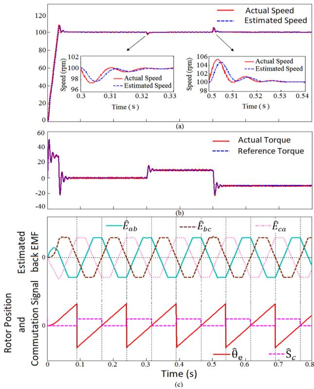
Fig. 10. Dynamic response of (a) speed (b) torque and (c) ZCP of back EMF, rotor position and commutation signal for step change in load torque from no-load to 10 Nm and from 10 Nm to -10 Nm with reference speed set at 100 rpm.
