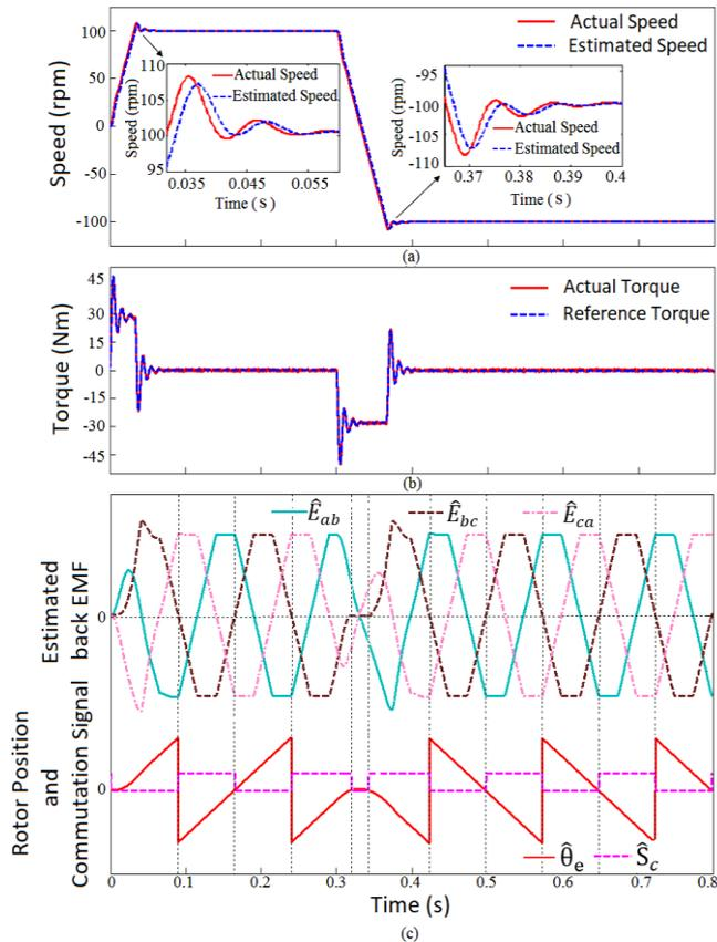
Fig. 7. Dynamic response of (a) speed (b) torque and (c) ZCP of back EMF, rotor position and commutation signal for step change in speed from 100 rpm to -100 rpm.
