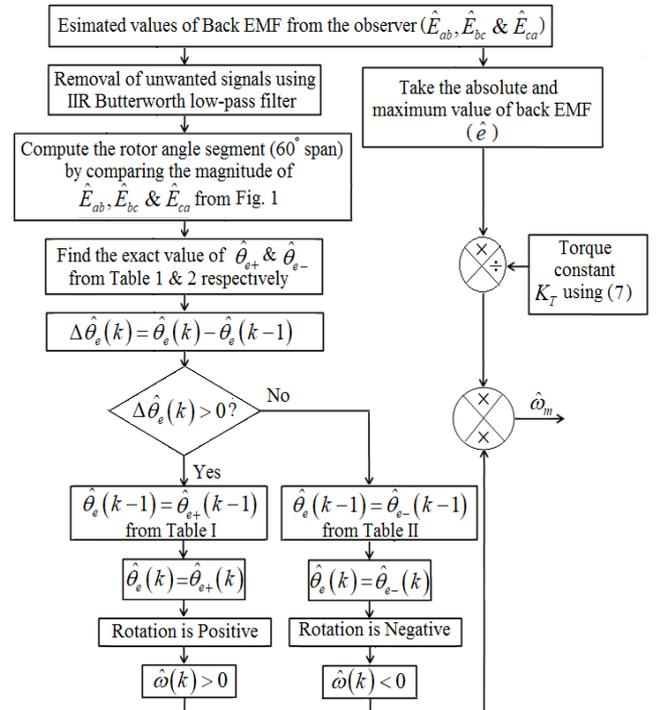
Fig. 3. Estimated speed algorithm for the BLDC motor.
