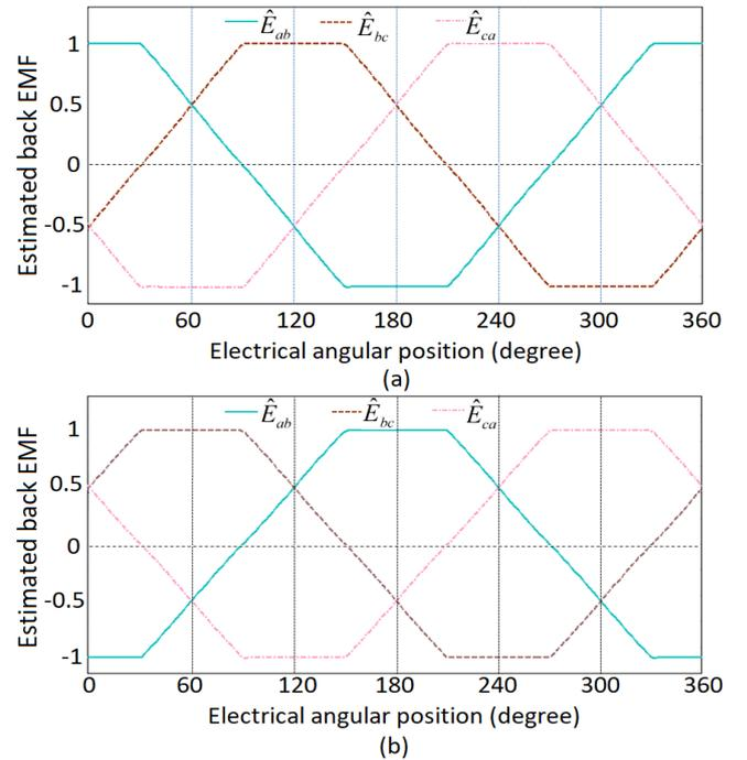
Fig. 1. Estimated back EMFs for (a) positive rotation and (b) negative rotation.
