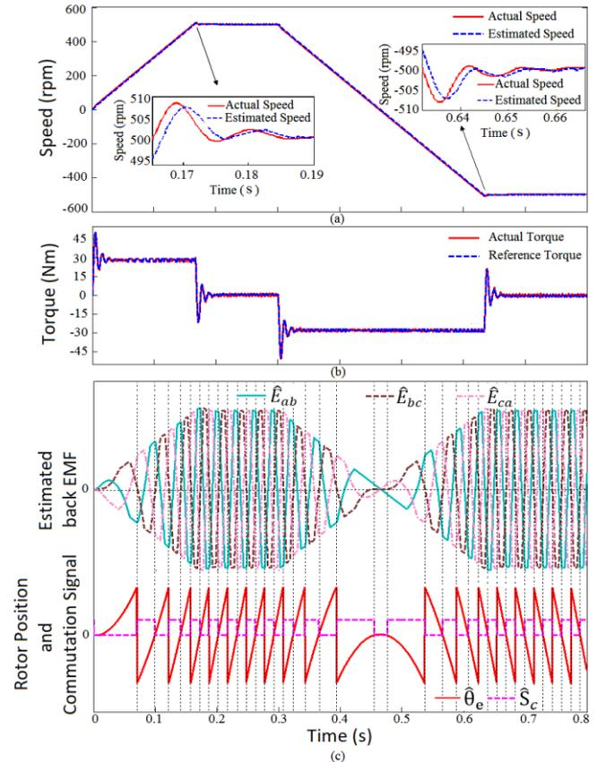
Fig. 8. Dynamic response of (a) speed (b) torque and (c) ZCP of back EMF, rotor position and commutation signal for step change in speed from 500 rpm to -500 rpm.
