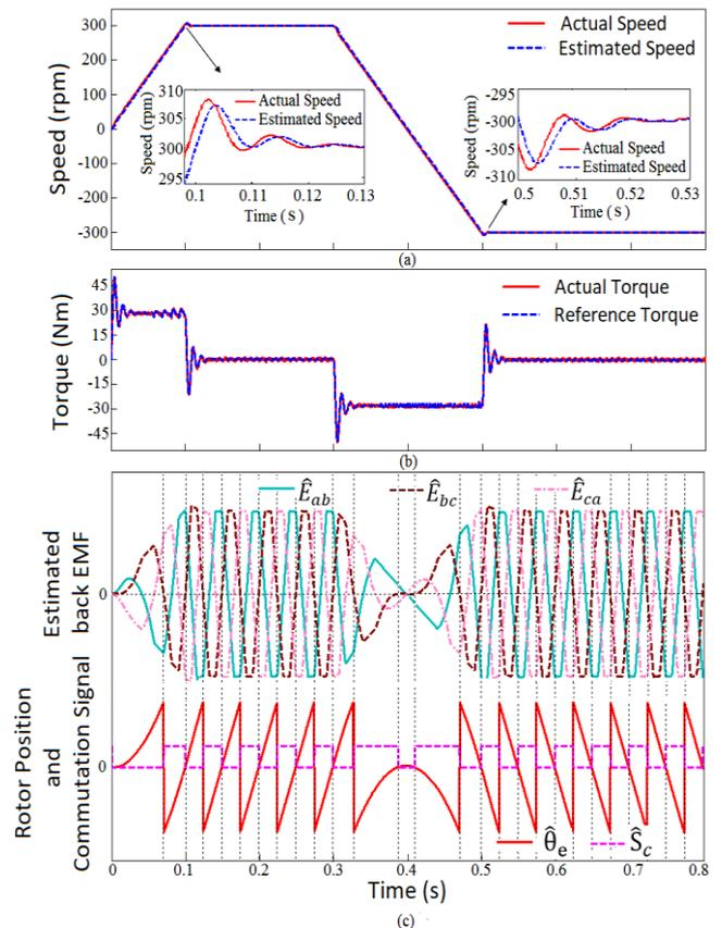
Fig. 6. Dynamic response of (a) speed (b) torque and (c) ZCP of back EMF, rotor position and commutation signal for step change in speed from 300 rpm to -300 rpm.
