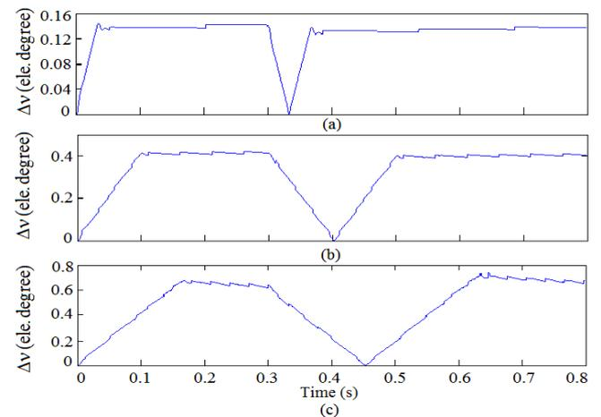
Fig. 12. Estimated rotor position error on no-load when step change in speed from (a) 100 rpm to -100 rpm (b) 300 rpm to -300 rpm and (c) 500 rpm to -500 rpm.
