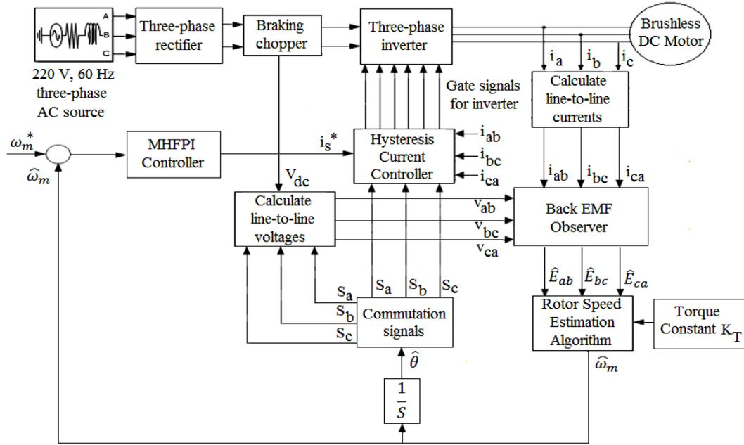
Fig. 4. Block diagram of the proposed sensorless BLDC motor.
