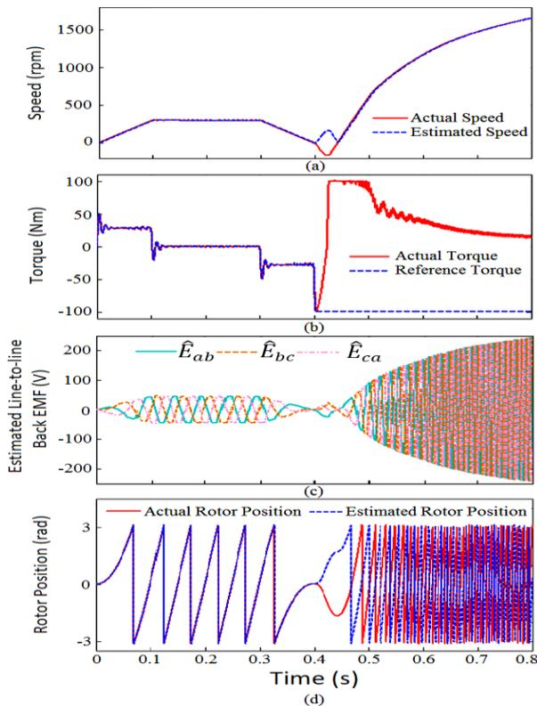
Fig. 5. Dynamic response of the BLDC motor for different step changes in reference speed.
