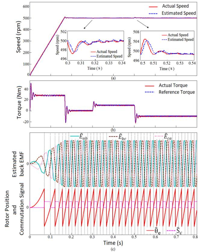
Fig. 11. Dynamic response of (a) speed (b) torque and (c) ZCP of back EMF, rotor position and commutation signal for step change in load torque from no-load to 10 Nm and from 10 Nm to -10 Nm with reference speed set at 500 rpm.
