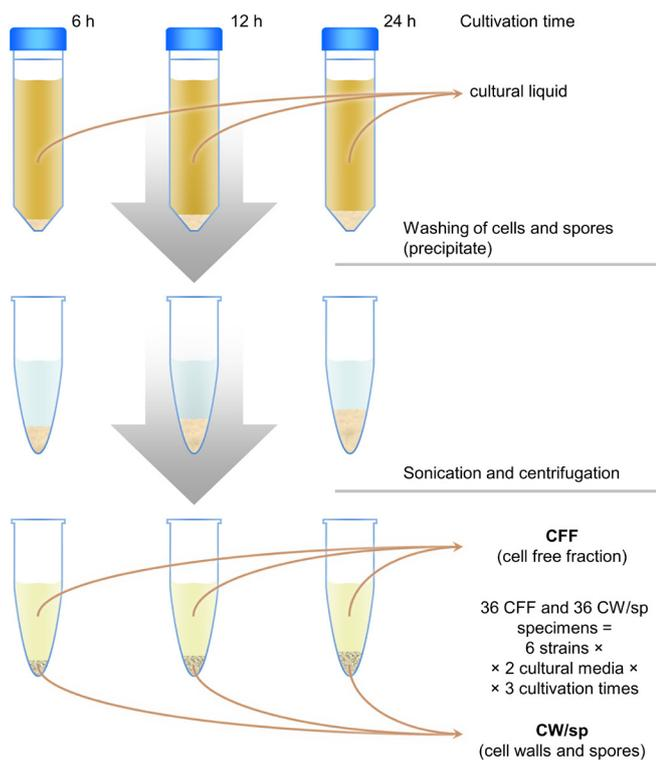
**Figure 1.** Scheme of obtaining CFF and CW/sp specimens.
