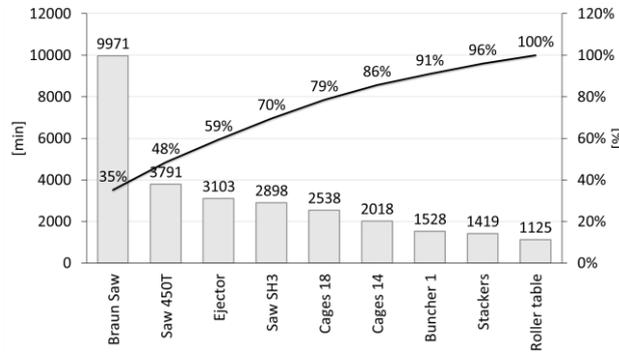
Fig. 1. Pareto analysis for individual devices at the rolling mill
