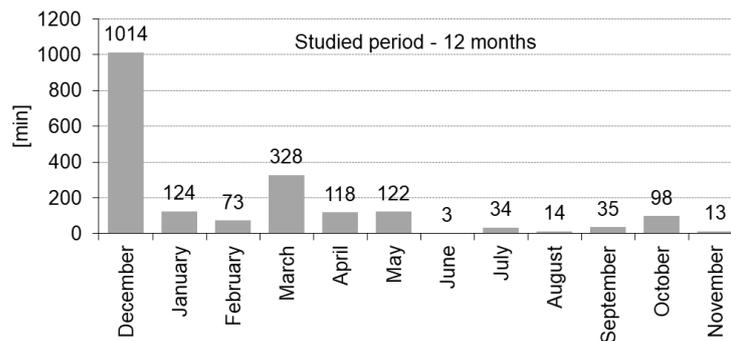
Fig. 3. Effect of implementing preventive actions for the N450 shear
