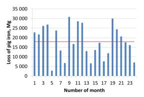
Fig. 3. The amount of loss of pig iron in the study period Source: (Information materials, 2018).
