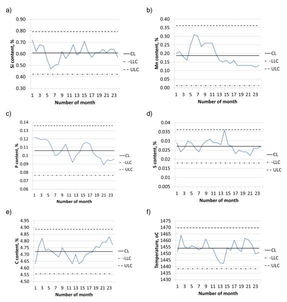
Fig. 1. Analysis of content of chemical elements and temperature of pig iron in the study period: a) Si content, b) Mn content, c) P content, d) S content, e) C content, f) temperature Source: (Information materials, 2018).
