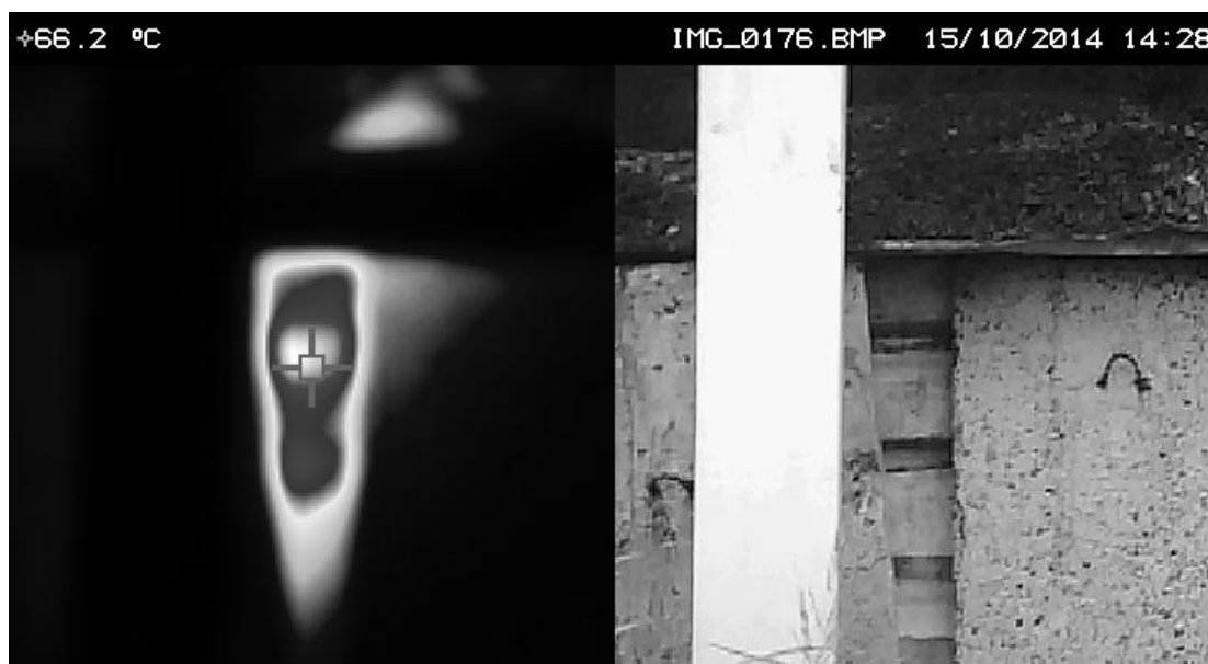
Fig.4. Thermal image indicating the rise of temperature of stored coal in place of damaged retaining wall (Author: Bogdan Sobociński)
