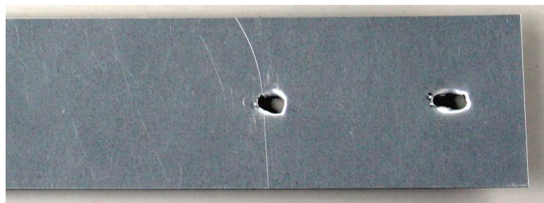
Fig. 3. Example of a connection bearing failure
