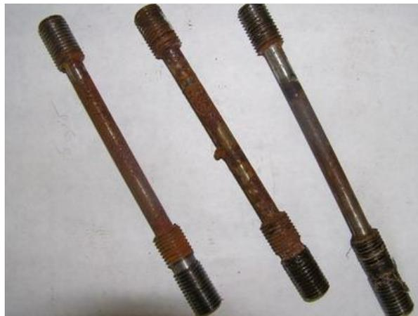
Fig. 5. Tested specimens for corrosion cracking with a welded rod
