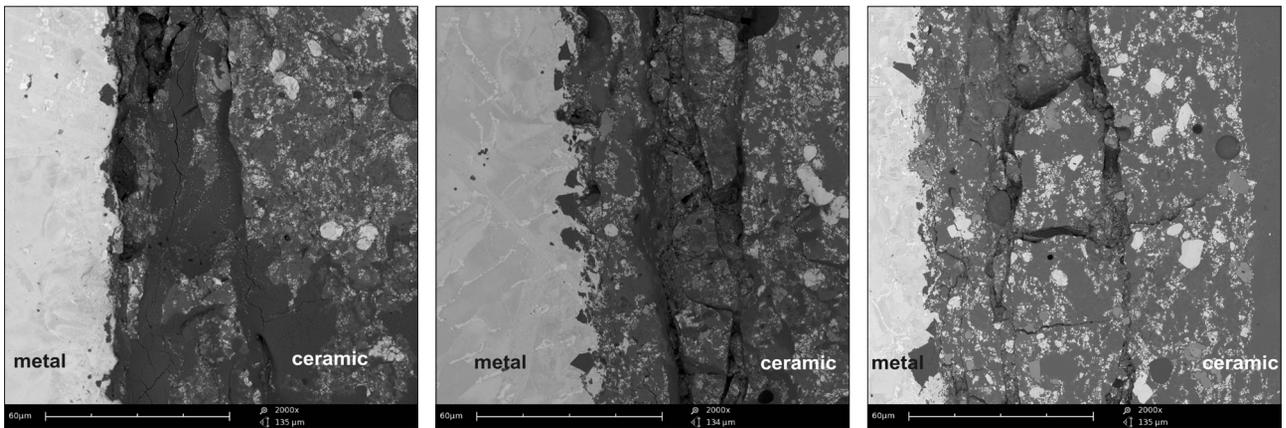
**Figure 5.** Microscopic SEM image of cross sections of metal-ceramics after adhesion testing for: (a) C1 castings made in 100% from the new factory material, (b) C2 castings made with 50% addition of recast material – cast once, (C) C3 castings made with 50% addition of recast material – cast twice.
