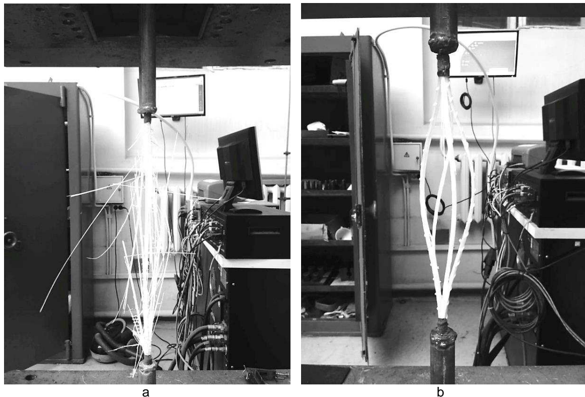
Fig. 2: Type of samples destruction caused by axial tension.
