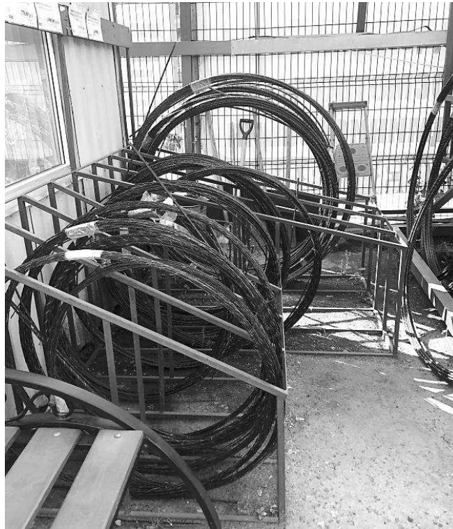
Fig. 1: Example of season storage of GFRP rebars in a warehouse.
