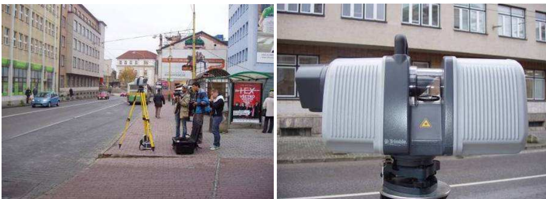
Fig. 7: The Trimble CX instrument during the road surface measurement of the public bus stop “Hurbanova” in Žilina on 22 October 2015.
