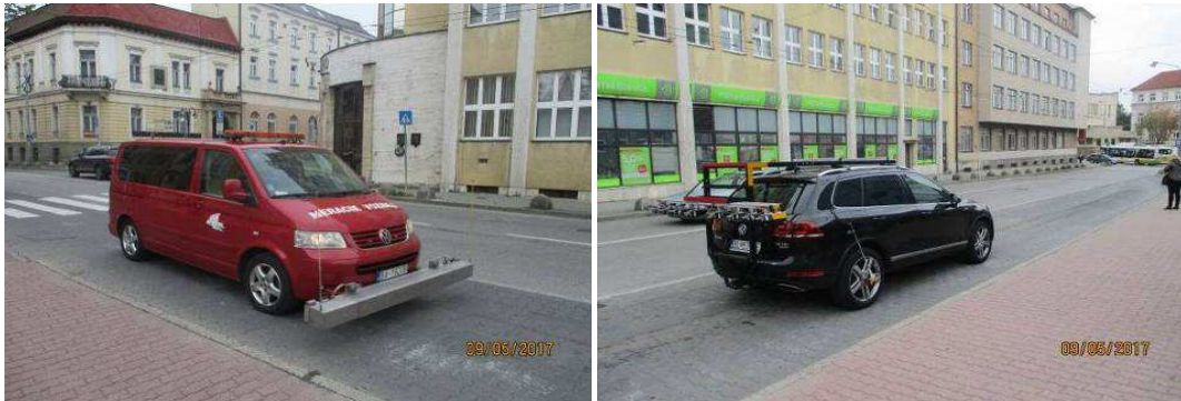
Fig. 6: View of measuring instrument Profilograph GE and Dynamic Road Scanner in measuring road surface morphology at the public bus stop “Hurbanova” in Žilina on 9 May 2017.
