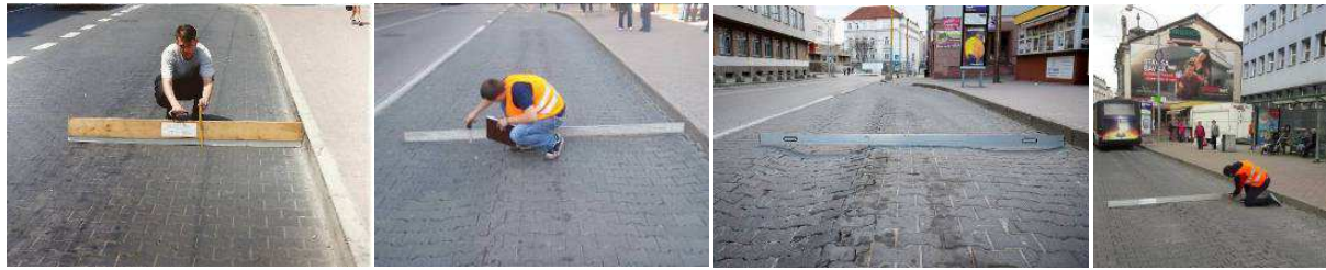
Fig. 12: Views of measurement process for determination of rut depth after the run of 160 000 design axles (DA) – on 27 August 1994, in the year 2012 after N_{AD} = 3.4 \cdot 10^6 , 2012, 2015 after N_{DA} = 4 \cdot 10^6 (Centre) and after N_{DA} = 4.5 \cdot 10^6 .
