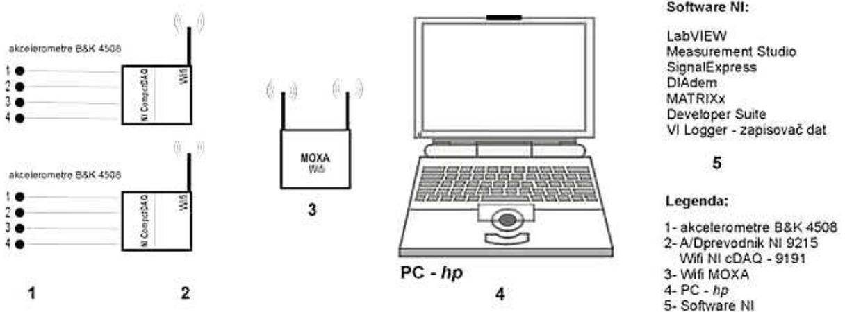
Fig. 6: Scheme of the measuring and the evaluation line.
