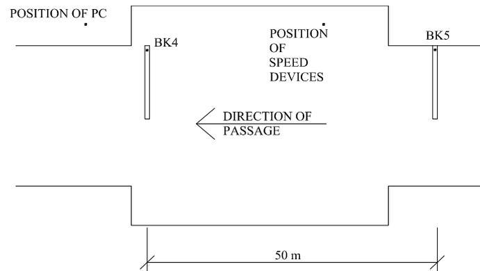
Fig. 2: Situation of the experimental track and the accelerometers on the pavement.
