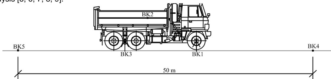
Fig. 1: Position of the accelerometers.
