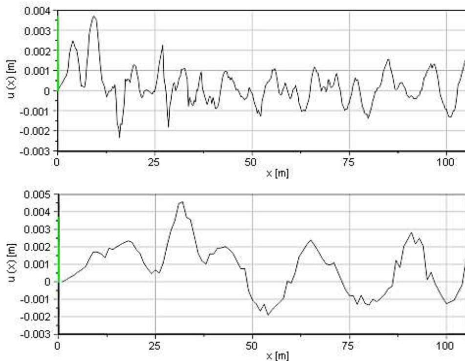
Fig. 7: Scanned profile of the test track under the tyre lines, left tyre line (above), right tyre line (below).
