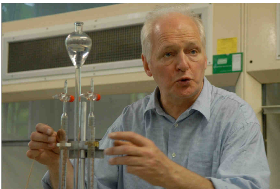
Fig. 7. The Hofmann Voltameter (1866) shows one of the most significant experiments of the 19th century - this is the decomposition of water (which for centuries had been considered to be an element) into hydrogen and oxygen
