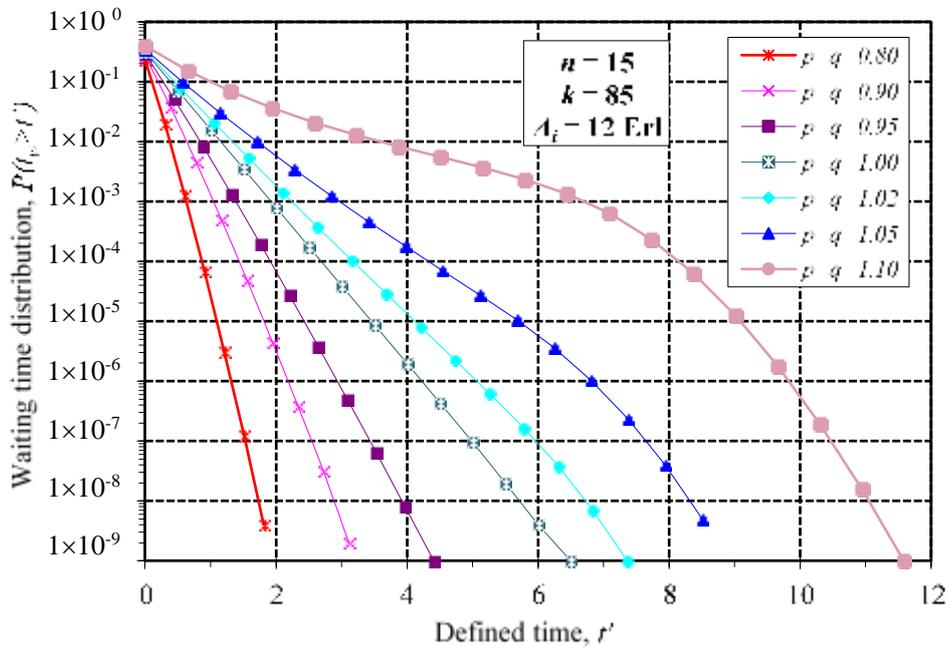
Fig. 14.  $M(g)/M(g)/n/k$  – Probability of waiting time exceeding the define time interval  $t'$ , as a function of  $t'$ , for different values of arrival and service peakedness factors  $p$  and  $q$  ( $n=15, k=85, A_i=12$  Erl)
