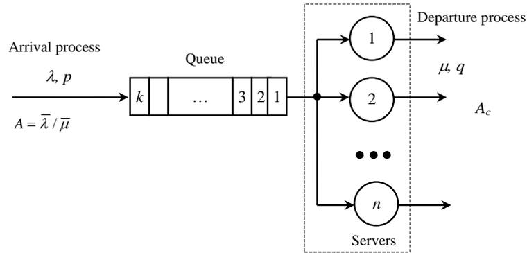
Fig. 3. A generalized multi-server queue –  $M(g)/M(g)/n/k$
