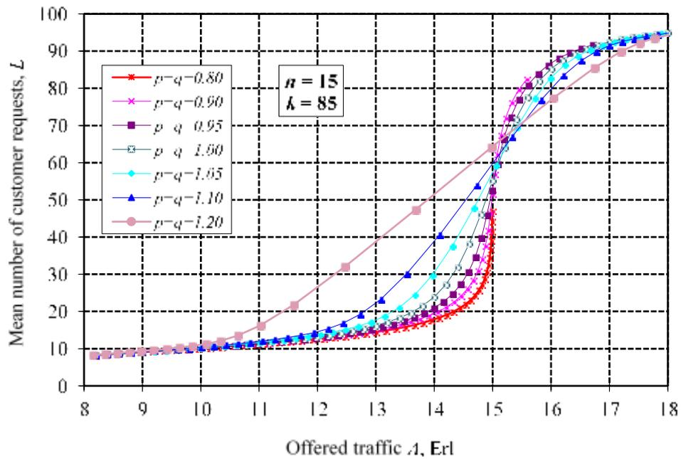
Fig. 12.  $M(g)/M(g)/n/k$  – Mean number of customer requests in the system as a function of the offered traffic, for different values of arrival and service peakedness factors  $p$  and  $q$  ( $n=15, k=85$ )
