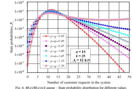
Fig. 6. M(g)/M(g)/n/k queue – State probability distribution for different value of peakedness factors p and q (n=15, k=35, A<sub>i</sub>=12 Erl)
