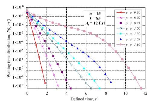
Fig. 14. M(g)/M(g)/n/k – Probability of waiting time exceeding the define time interval t', as a function of t', for different values of arrival and service peakedness factors p and q (n=15, k=85, A\_i=12 Erl)
