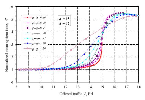
Fig. 13. M(g)/M(g)/n/k – Normalized mean system time as a function of the offered traffic, for different values of arrival and service peakedness factors *p* and *q* (*n*=15, *k*=85)
