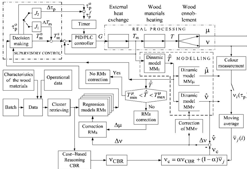
Fig. 6. Scheme of inference control of thermal treatment of wood materials, including CBR
