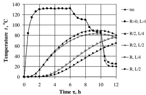
Fig. 3. Change in  $t_m$  and  $t$  in five characteristic points of the longitudinal section of beech log with  $D = 0.4$  m,  $L = 0.8$  m, and  $t_0 = 0$  °C during autoclave steaming and subsequent conditioning at 20 °C
