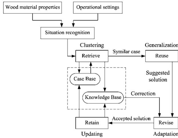
Fig. 7. Scheme of the  $R_c^4$  – CBR
