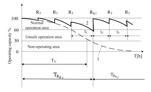
Figure no. 1 The scheme of executing technical interventiona in the planned preventive system 1 – The evolution curve of the technical condition in the absence of technical interventions 2 – The curve of the evolution of the technical state in the situation of performing the technical interventions
