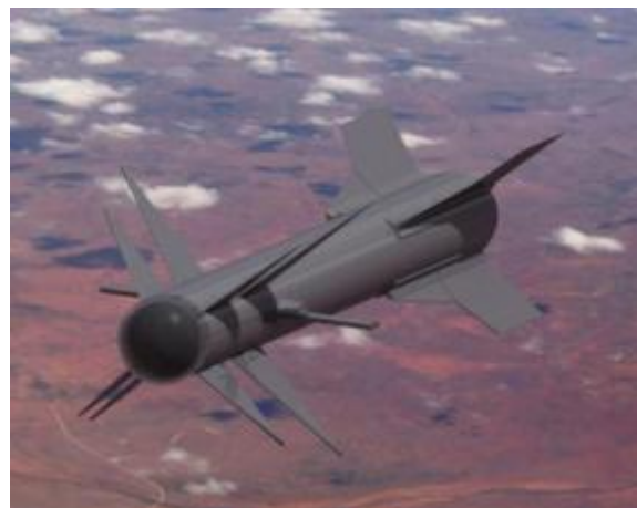
Figure no. 7. External configuration with command surfaces
