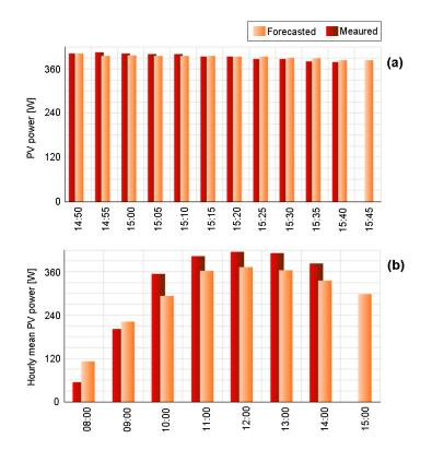
Fig. 4. Illustration of the PV-L system output power forecasting in August 20, 2018, at two time horizons (a) 5 minutes – instantaneous power is forecasted and (b) one hour – hourly average of the output power is forecasted.
