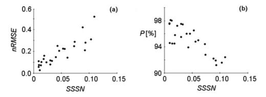
Fig. 2. Comparison between the SPN1 and SMP10 pyranometers to the measurement of: (a) global solar irradiance and (b) sunshine number as function of the daily average of sunshine stability number. nRMSE represents the root mean square error and P is the percentage of sunshine number measurements in which both pyranometers estimate the same value for sunshine number. Each point on the graphs corresponds to a day of May 2018.
