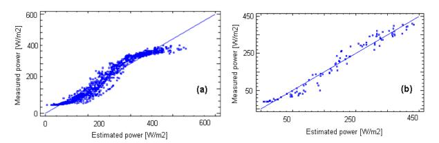
Fig. 3. Measured vs. estimated power delivered by the experimental system PV-L at two intervals of time: (a) instantaneous and (b) hourly mean. The graphs were built with data recorded during 7-20 June 2018.
