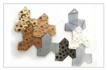
Fig. 6. CNC milled samples of plywood, pine and hardwood, water-jet cut marble slab with laser engraving, laser cut acrylic glass with laser engraving, sheet metal treated with acid through vinyl, white concrete cast in a CNC milled negative extruded polystyrene mold, and resin cast in a rubber mold. The concept of geometries is repeating displacement tessellation along hexagonal grid. Author: Ana Lucía Estrada Castillo, class of Spring 2018 [Figure: A.Riekstinš].
