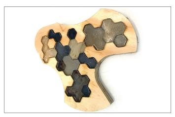
Fig. 11. Plywood milled in variable depth revealing its various dually dark and light layers of pine, filled with resin that is all in one uniform light blue color, but due to the different depth it has the quality of water that absorbs and scatters the white light. Author: Néstor Isaías Torres García, class of Spring 2018 [Figure: A.Riekstinš].
