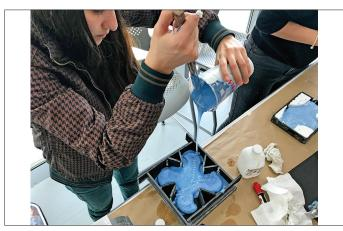
Fig. 9. Mold making with liquid silicone rubber in a foam board box over a solid MDF laser-cut piece. Author: Priscila Ramírez de los Santos, class of Spring 2018 [Figure: A.Riekstiņš].
